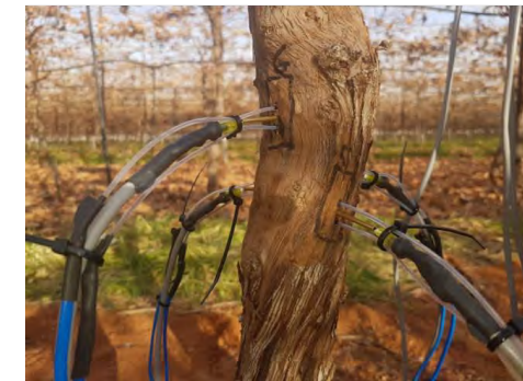
Sapflow monitoring (3 vines/sub-plot, probe depths 10, 15, 20, 25 mm)
